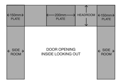
\*If an I-beam has been used in the head, it must be packed out with either brick, timber or plates to be welded (see diagram left) & flush on the plaster. This also applies to the side room (at least 150mm wide).
